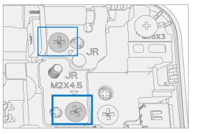
5. **Set AB-Cover Display Angle to 90 deg for Safe Removal** – Place the display module at an angle of about 90 degrees. Use a PH0 screwdriver to remove the 2 outer screws at the left and right hinges while holding the display with your free hand.
