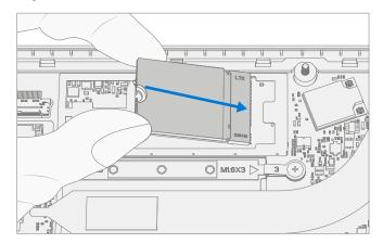
2. **Install new rSSD screw** – Using a PH00 screwdriver install a new MM16030I130 rSSD screw until the screw is just snug and seated, and then turned another 45 degrees (1/8 turn).
