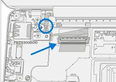
4. **Connect Antenna cable** – Carefully install two antenna connectors on the mainboard. Install a new clear Mylar shield over the antenna connectors. Secure the antenna cables to the D-Bucket with the supplied black tape.
