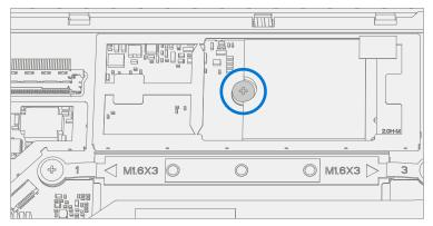
3. **Install SSD Shielding cover** – Install a new Shielding cover on Main board.
