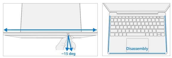
d. Gently rotate the opening tool at the hinge corner until you hear a soft pop from the snap. Repeat this for both hinges.
