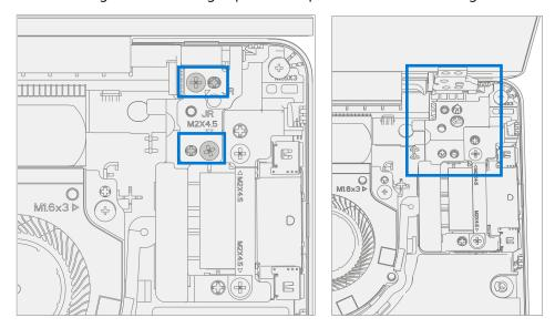
2. **Remove Bracket** – Use a PH0 screwdriver to remove 2 screws and a PH00 screwdriver to remove a 3rd screw securing the right bracket. Remove the bracket from the D-Bucket.
