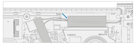
! CAUTION: Ensure the antenna with the shrink wrap ring is connected to the top interface.
