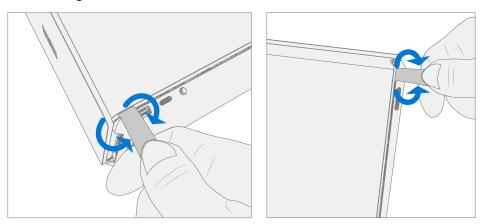
e. To disengage the 4 vent snaps, ensure the device is open to 90 degrees and the display is lying flat on the work surface. Gently push the C-Cover downward towards the work surface and rotate it for towards the screen.
