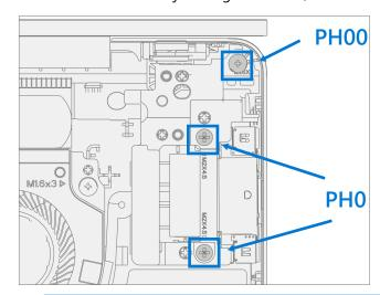
! CAUTION: Ensure the antenna cables are routed under the tab on the bracket.
