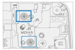
2. **Install Two Inner Hinge Screws** – Using a PH0 screwdriver, install 2 new inner MM200481000 screws on the left and right hinges. Screws should be installed until just snug and seated, and then turned another 90 degrees (1/4 turn).
