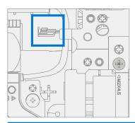
3. **Install Right AB-Cover hinge Screws** – Tilt the hinge down over the right bracket. Use a PH0 screwdriver to install one MS20055I430 screw, and one MM20048I000 screw into the AB-Cover hinge. Screws should be installed until just snug and seated, and then turned another 45 degrees (1/8 turn).
