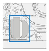
2. **Install Bracket** – Place right bracket in the D-Bucket over the Surflink. Use a PH0 screwdriver to install 2 new MM20045I080 screws and a PH00 screwdriver to a new MM16030I130 screw into the right bracket. Screws should be installed until just snug and seated, and then turned another 45 degrees (1/8 turn).
