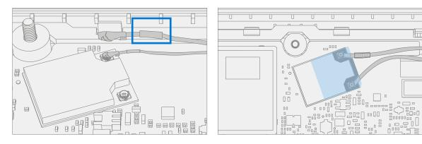
! CAUTION: Ensure the antenna cables are routed under the tab on the bracket near the hinge.
