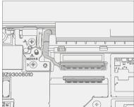
4. **Remove Two Inner Hinge Screws** – Use a PH0 screwdriver to remove the 2 inner screws on the left and right hinges.
