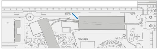
3. **Disconnect Display connector** – Lift up on the metal buckle. Then slide out the Display connector from the Mainboard connector.
