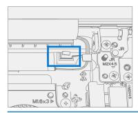
5. **Install Thermal Module (Heatsink)** – Gently clean off the residual thermal grease from the two IC chips with a lint free cloth. Make sure there are no contaminants or residual grease. Check that the thermal grease on the underside of the new thermal module is intact and not smeared. Place the thermal module over the two IC chips. Using a PH00 screwdriver Install 4 new MM16030I130 screws until just snug and seated, and then turn another 45 degrees (1/8 turn).
