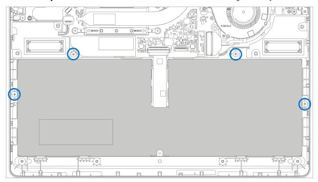
2. **Remove Battery** – Carefully lift battery up and out of the D-Bucket.
