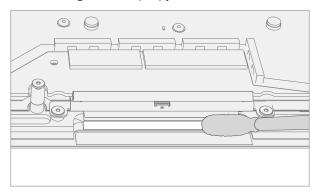
c. **Install New Display Cable Foam** – Remove the liner from the display cable foam. Align the display cable foam adhesive side down onto the Keyboard over the silver surface. Press down on the foam for 30 seconds. Repeat this for each side of the Keyboard.
