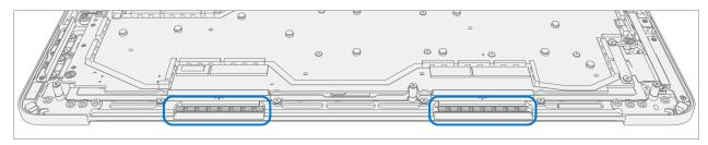
a. **Remove left and right foam** – Using a plastic tool remove the display cable foam from the left and right sides of the Keyboard.
