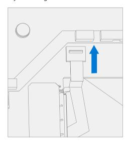
13. **Connect Keyset FPC** – Ensure the lock is released on the Keyset FPC connector. Install the Keyset FPC into the PCBA connector. Secure the connector lock.
