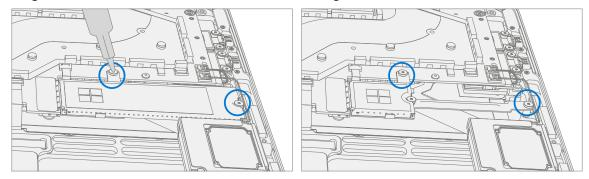
b. Pull the rSSD out of the motherboard connector.
