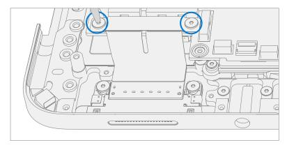
5. **Install Left I/O Bracket** – Place the left I/O bracket onto the Keyboard. Using a 3IP (Torx-Plus) driver install 3 new Left I/O Bracket Screws (M1109237). Turn all screws until just snug and seated, and then turn another 45 degrees (1/8 turn) or until fully fastened.
