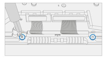
d. Using a pair of tweezers apply foam to the connector cable in area shown.
