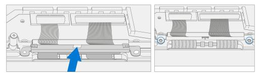
b. Ensure that the cables route over the plastic guide along the edge of the motherboard.
