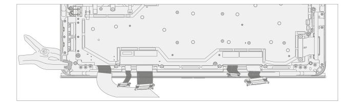
11. **Pre-fasten right hinge screws** – Assemble 4 new Hinge Screws (M1150078) in the right-side hinge and tighten until just snug.
