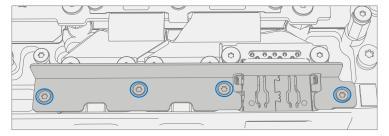
12. **Remove USB Bracket** – Using a 3IP (Torx-Plus) driver remove the 3 screws securing the USB Bracket to the motherboard.
