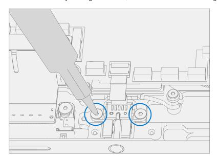
4. **Install Left I/O Bracket** – Place the left I/O bracket onto the Keyboard. Using a 3IP (Torx-Plus) driver install 3 new Left I/O Bracket Screws (M1109237). Turn all screws until just snug and seated, and then turn another 45 degrees (1/8 turn) or until fully fastened.
