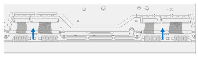
a. Ensure that the cables route over the plastic guide along the edge of the motherboard.
