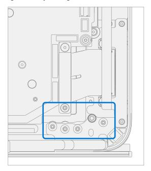
12. **Pre-fasten left hinge screws** – Remove the 1-inch light duty clamp form the left hinge. Assemble 4 new Hing Screws (M1150078) in the left side hinge and tighten until just snug.
