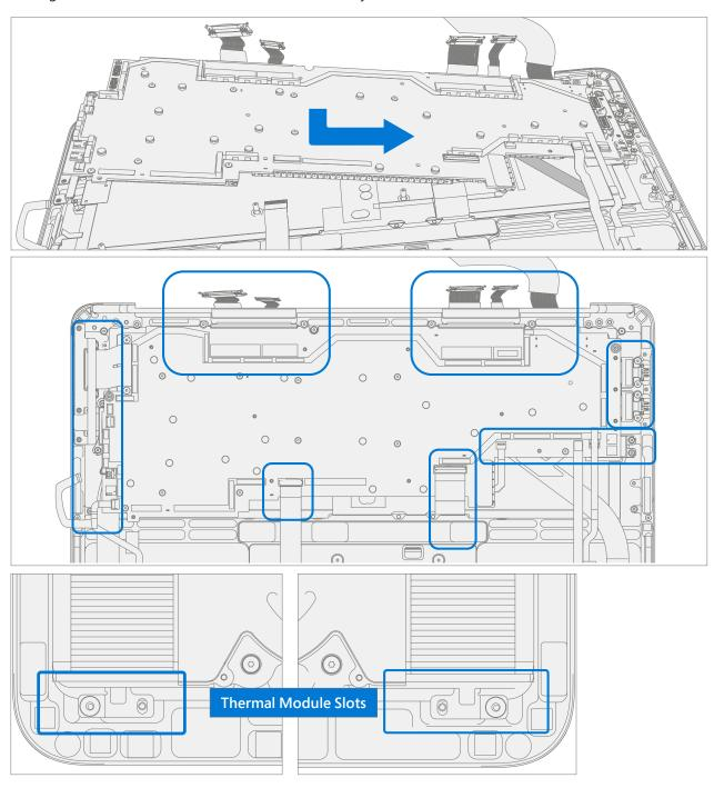
**IMPORTANT:** Verify the 15 cables and FPC's are not captured under the PCBA. The Fan and Wireless Pen Charger FPCs route over the thermal heat pipe. Ensure the thermal module slots align over the posts in the Keyboard.
