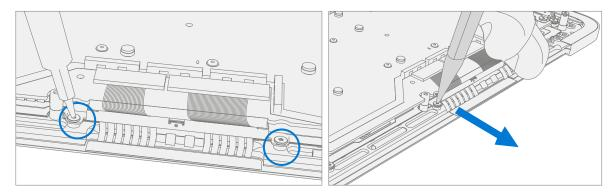
2. **Disconnect 4 Display Cables** – Use plastic tool to unlatch the connectors on the 4 display cables and carefully remove the cables from the PCBA connectors.
