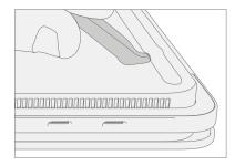
2. **Cleaning** – Remove any adhesive tape remnants from the chassis and clean off any glue residue with 70% or greater Isopropyl Alcohol.
