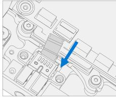
5. **Disconnect 4 Speaker Cables** – Using a plastic tool carefully release the 4 speaker connectors from the PCBA.
