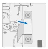
3. **Connect Left Tweeter** – Connect the left tweeter to the motherboard by aligning with connector and pressing down firmly.
