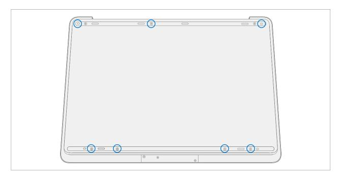
2. **Mark Tool Pick Depth** – To prevent damage to internal components use a metric ruler to draw a 13 mm mark on two plastic picks.
