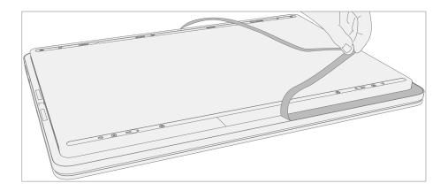
**IMPORTANT:** Along the front edge pull the cosmetic plate in a tight 'U' shape to prevent the pen shim from lifting with the cosmetic plate. A replacement pen shim is included with the new Cosmetic Plate in situations where it is removed.
