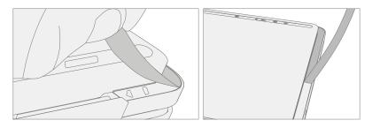
**IMPORTANT:** Pull the cosmetic plate away from the device at an angle to prevent scratching the Chassis.
