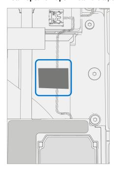
10. **Connect 4 Speaker Cables** – Align the left and right Speaker Cable connectors to the PCBA and press down. Ensure the cables do not overlap and are routed as pictured below.
