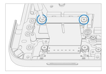
3. **Disconnect Surflink FPCs** – Using a plastic tool disconnect the Surflink FPCs from the PCBA.
