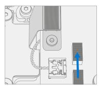
3. **Disconnect Micro SD FPC** – Use a plastic spudger to disconnect the Micro SD FPC from the motherboard.
