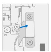
7. **Install Micro SD Slot Bracket** – Place the Micro SD Bracket over the FPC. Using a 3IP (Torx-Plus) driver, install the 2 Micro SD Bracket Screws (M1156309). Turn all screws until just snug and seated, and then turn another 45 degrees (1/8 turn) or until fully fastened.
