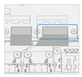
3. **Install USB Bracket** – Install the USB bracket using 3IP (Torx-Plus) driver and 3 USB Bracket Screws (M1167780). Turn all screws until just snug and seated, and then turn another 45 degrees (1/8 turn) or until fully fastened.
