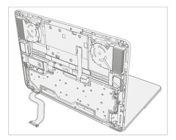
5. **Remove Left Hinge Screws** – Using a 6IP (Torx-Plus) driver remove the 4 screws on the left hinge. Apply a 1 inch light duty spring clamp to the left hinge to hold it in place against the C-Cover.
