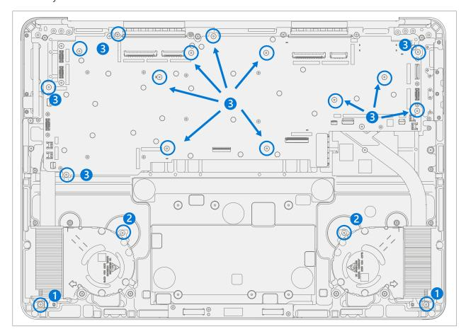
19. **Remove Fans** – Remove the left and right fans from the chassis. Reserve the grommets under the fans for future installation.
