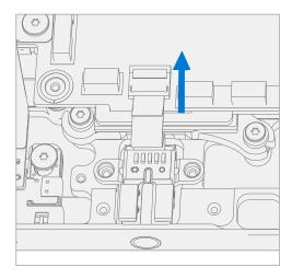
18. **Connect Surflink FPCs** – Align the FPC's connectors to the PCBA and press down.
