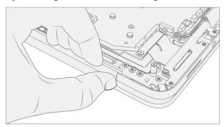
d. Verify a 0.2 mm plastic thickness gauge can slide easily in the hinge gap.
