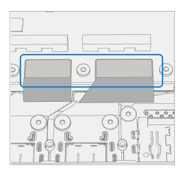
5. **Install USB Bracket**– Install the USB bracket using 3IP (Torx-Plus) driver and 3 USB Bracket Screws (M1167780). Turn all screws until just snug and seated, and then turn another 45 degrees (1/8 turn) or until fully fastened.
