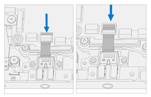
3. **Install New Audio Jack Screws** – Using a 3IP (Torx-Plus) driver install 2 new Audio Jack Screws (M1168360). Turn all screws until just snug and seated, and then turn another 45 degrees (1/8 turn) or until fully fastened.
