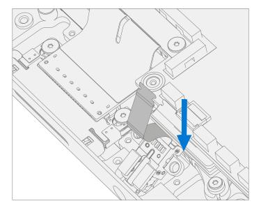
2. **Connect Audio Jack FPC** – Ensure the lock is released on the Audio Jack FPC connector. Install the Audio Jack FPC into the PCBA connector. Secure the connector lock.
