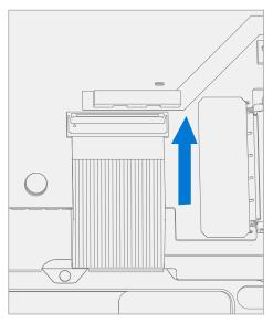
14. **Connect Trackpad FPC** – Ensure the lock is released on the Trackpad FPC connector. Install the Trackpad FPC into the PCBA connector. Secure the connector lock.
