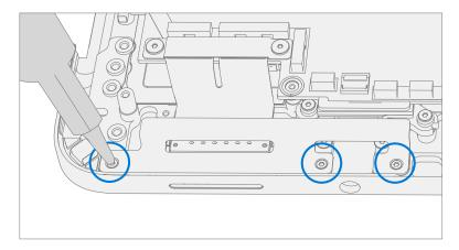
2. **Remove Audio Jack Screws** – Using a 3IP (Torx-Plus) driver remove the 2 screws securing the audio jack to the Keyboard.
