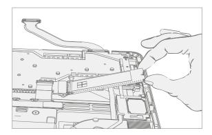
8. **Install new rSSD screws** – Using a 3IP (Torx-Plus) driver install 2 new rSSD Screws (M1167371). Turn all screws until just snug and seated, and then turn another 45 degrees (1/8 turn) or until fully fastened.
