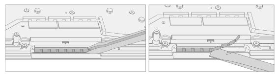
b. **Cleaning** – Remove any adhesive tape remnants from the Keyboard and clean off any glue residue with 70% or greater Isopropyl Alcohol.
