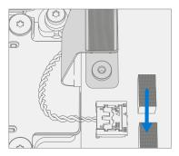
4. **Install Bracket** – Place the Micro SD Bracket over the FPC. Using a 3IP (Torx-Plus) driver, install the 2 Micro SD Bracket Screws (M1156309). Turn all screws until just snug and seated, and then turn another 45 degrees (1/8 turn) or until fully fastened.
