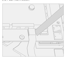
11. **Remove Fan FPC Tapes** – Carefully remove the 4 black tapes securing the fan FPCs. And 1 black tape securing the subwoofer.
