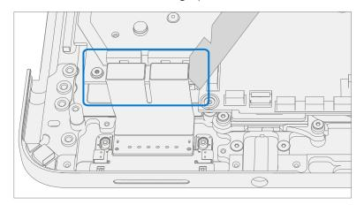
5. **Remove Surflink Port** – Remove the Surflink Port from the Keyboard.
