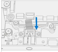
4. **Remove Audio Jack** – Remove the audio jack from the Keyboard by pulling up on the side with the FPC. Carefully move the Audio Jack from side to side during removal.
