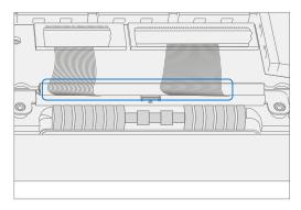
c. Using a 3IP (Torx-Plus) driver install the 2 new Tensioner Screws (M1177566) in each cable tensioner. Turn each screw until just snug and seated, and then turn another 45 degrees (1/8 turn) or until screws are fully fastened.
