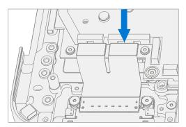
19. **Install Surflink Bracket** – Place the bracket over the Surflink FPCs. Using a 3IP (Torx-Plus) driver install 2 new Surflink Bracket Screws (M1149393). Turn all screws until just snug and seated, and then turn another 45 degrees (1/8 turn) or until fully fastened.
