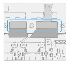
16. **Remove Micro SD Slot Bracket** – Use a 3IP (Torx-Plus) driver to remove the 2 Micro SD Bracket Screws and remove the bracket.
