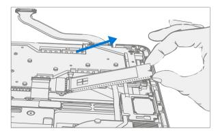
c. **Remove Thermal Pad** – Remove old rSSD thermal pad and clean residue with IPA.
