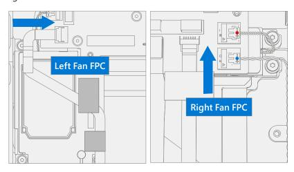
16. **Install New Fan FPC Tapes** – Refer to the picture below for tape locations. Apply 2 black tapes to the left Fan FPC securing it to the left speaker. Apply 1 black tape on the right Fan FPC securing it to the right speaker. Apply 1 black tape on the right Fan FPC securing it to the Keyboard.
