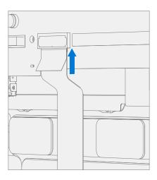
15. **Connect Fan FPCs** – Ensure the locks are released on the left and right Fan FPC connectors. Install the left and right Fan FPCs into the PCBA connectors. Secure the connector locks.
