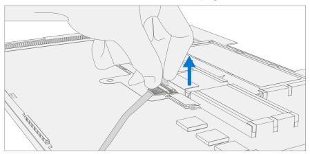
b. Using the "Pull" tab, slide the connector carefully towards the battery to release the latches and remove the cable. Avoid impacting or poking the battery during this process.
