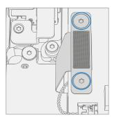
17. **Disconnect Micro SD FPC** – Use a plastic spudger to disconnect the Micro SD FPC from the motherboard.
