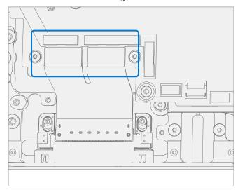
3. **Install new Surflink Port screws** – Using a 3IP (Torx-Plus) driver install 2 new Surflink Screws (M1149393). Turn all screws until just snug and seated, and then turn another 45 degrees (1/8 turn) or until fully fastened.
