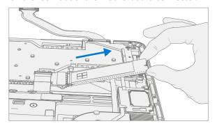
2. **Remove 2230 rSSD from bracket** – Using a 3IP (Torx-Plus) driver remove the screw securing the 2230 rSSD to the bracket and then remove the rSSD.
