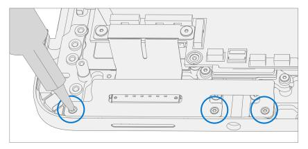
2. **Remove Surflink Bracket** – Using a 3IP (Torx-Plus) driver remove the 2 screws securing the Surflink Bracket to the PCBA. Remove the cable retainer.
