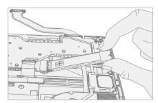
4. **Install new rSSD screws** – Using a 3IP (Torx-Plus) driver install 2 new rSSD Screws (M1167371). Turn all screws until just snug and seated, and then turn another 45 degrees (1/8 turn) or until fully fastened.
