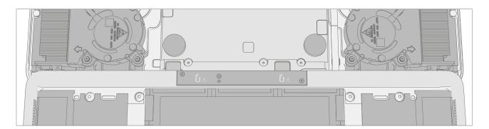
9. **Remove Pen Shim (Optional)** – If pen shim was damaged during the removal of the cosmetic plate it must be replaced. On the Keyboard Assembly place the pointed end of a spudger underneath the right side of the shim to pry it up and remove it. Clean any residual PSA with IPA.
