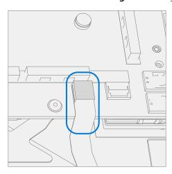
12. **Connect Keyset Backlight FPC** – Ensure the lock is released on the Keyset Backlight FPC connector. Install the Keyset Backlight FPC into the PCBA connector. Secure the connector lock.
