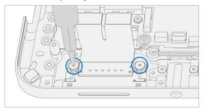
4. **Install Surflink Bracket** – Place the bracket over the Surflink FPCs. Using a 3IP (Torx-Plus) driver install 2 new Surflink Screws (M1149393). Turn all screws until just snug and seated, and then turn another 45 degrees (1/8 turn) or until fully fastened.
