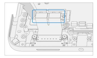
4. **Disconnect Audio Jack FPC** – Release the lock on the Audio Jack FPC connector. Remove the Audio Jack FPC from the PCBA connector.
