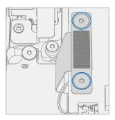
8. **Install Left and Right Speakers** – Place the left and right speakers into the Keyboard. Using a 3IP (Torx-Plus) driver install 3 new Speaker Screws (M1202147) in the left speaker, and 3 new Speaker Screws (M1202147) in the right speaker. Turn all screws until just snug and seated, and then turn another 45 degrees (1/8 turn) or until fully fastened.
