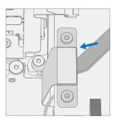
4. **Remove Micro SD Slot** – Using a 3IP (Torx-Plus) driver remove the 2 SD Slot Screws from the chassis. Lift Micro SD Slot to remove.
