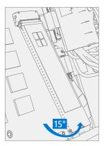
2. **Install rSSD screw** – Using a 3IP (Torx-plus) driver install the rSSD screw. Turn until just snug and seated, and then turn another 45 degrees (1/8 turn) or until fully fastened.
